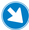
D2 Instruction to all drivers to keep to the right of the sign (or left if arrow is reversed)
