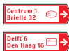
K7 Signposts for cyclists and moped riders (finger posts) showing local and intermediary destinations, municipal cycle route numbers (above) and showing intermediary destinations and intermediary cycle route numbers (below)
